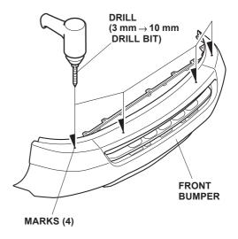
While wearing eye protection, drill a 3 mm hole through four dimpled areas of the front bumper on both sides. Remove any burrs from the edges of the holes with a file.
