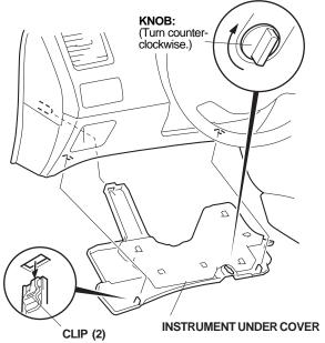
14. Release the eight clips, and remove the instrument lower cover by pulling it toward you. Take care not to damage the clips.
