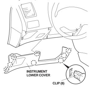
15. Release the four clips, and remove the assistant lower cover by pulling it toward you. Take care not to damage the clips and pins.
