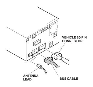
43. Connect the four vehicle connectors to the center panel, and reinstall the center panel.
