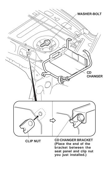
39. Slide the two clip nuts onto the CD changer brackets and parcel shelf through the holes in the parcel shelf, and align their holes as shown. Install the two washer-bolts, and tighten them securely.
