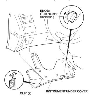
14. Release the eight clips, and remove the instrument lower cover by pulling it toward you. Take care not to damage the clips.
