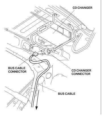
41. Fold the excess BUS cable and secure the BUS cable to the holes of the rear seat panel with the two wire ties with clip.
