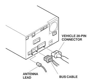
43. Connect the four vehicle connectors to the center panel, and reinstall the center panel.
