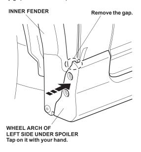
Loosely install the front self-tapping screws in the holes in the wheel arch of the left side under spoiler.
