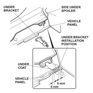
22. Cut into the marked area of the under coat with a utility knife, and file off the under coat from the surface side and inner side of the vehicle panel.
