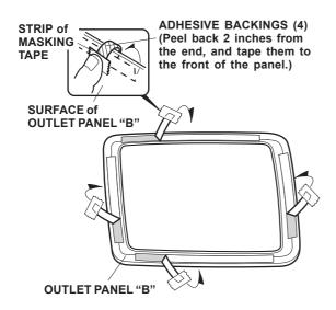
10. Position the outlet panels "A" and "B" on the existing outlet panels. While holding pressure on the outlet panels, carefully remove the adhesive backings from the outlet panels. Hold the outlet panels "A" and "B" firmly against the existing outlet panels with the palm of your hand, particularly at the edges.
