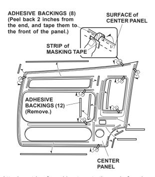
5. Attach a strip of masking tape to the end of each shaded adhesive backing. Peel back 2 in. (5 to 6 cm) of the adhesive backings and fold them over as shown. Temporarily attach the strips of masking tape to the outside of the center panel. Remove all remaining adhesive backings from the center panel.
