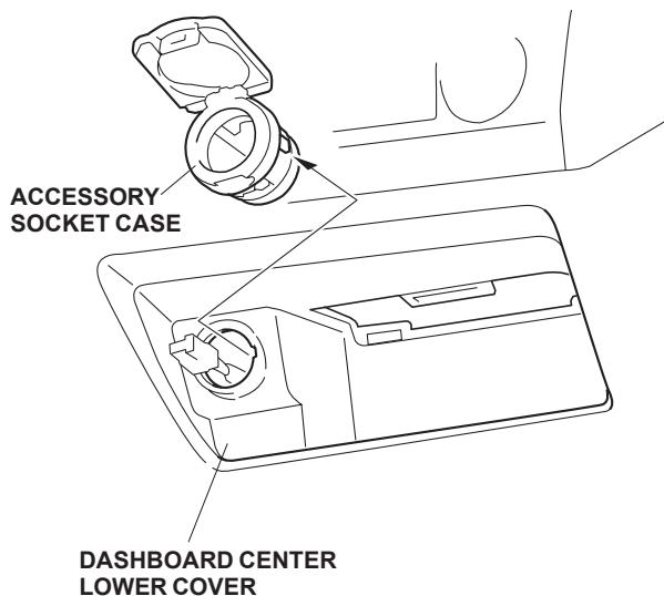
7. Slide the ring into the hole in the dashboard center lower cover in the direction shown.
