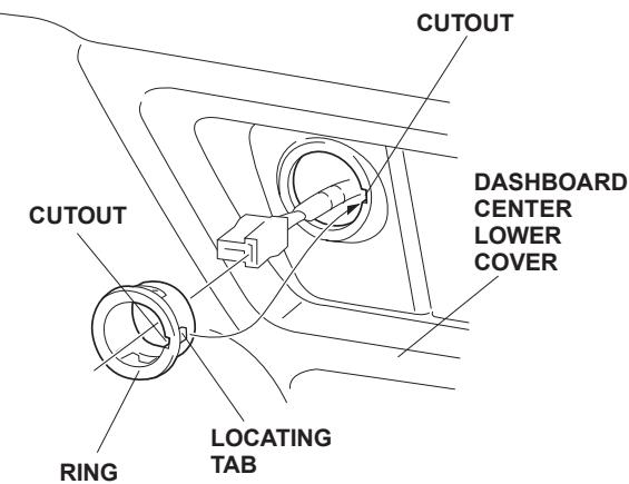
8. Connect the vehicle 2-pin connector to the socket.
