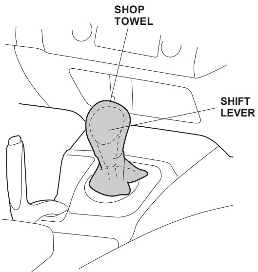
4. Shift to "S" or "2." Remove the lid from the dashboard center lower cover (four retaining tabs).
