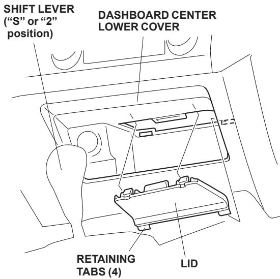
5. Open the accessory socket cover. Using a shop towel around a small flat-tip screwdriver, gently pry on the accessory socket to pop it out. Disconnect the vehicle 2-pin connector from the accessory socket.
