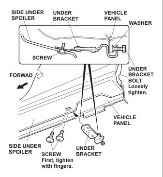
30. Position the under bracket on the side under spoiler and loosely install the two screws. Tighten the under bracket bolt, but don't tighten it completely yet.
