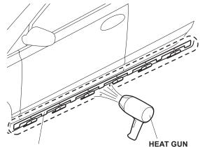
SIDE LOWER BRACKET Warm up the side lower bracket when the workshop room temperature is below 60°F(15°C).
