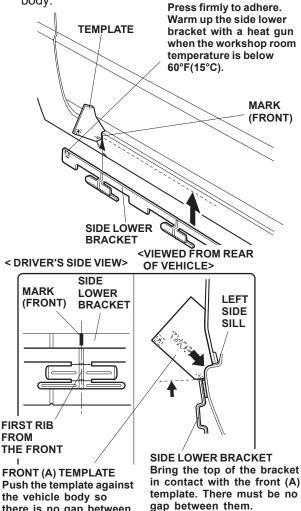
body. 12. Press the front end of the side lower bracket (where you removed the adhesive backing) to adhere the part firmly to the vehicle body.
