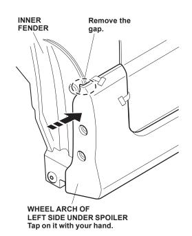
28. Loosely install the front self-tapping screws in the holes on the wheel arch of the left side under spoiler.
