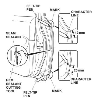
Position the hem sealant cutting tool against the door edge, and trim the seam sealant from mark to mark.
