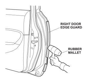
7. Repeat steps 3 through 6 to install the left door edge guard on the left front door.
