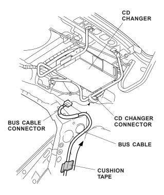
38. Fold the excess BUS cable, and secure the BUS cable to the holes in the rear seat panel with the two wire ties with clips.
