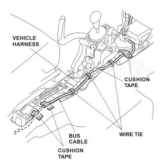
25. Using isopropyl alcohol on a shop towel, clean the areas where the cushion tape will attach. Attach the BUS cable to the floor panel with the three cushion tapes in the area shown.
