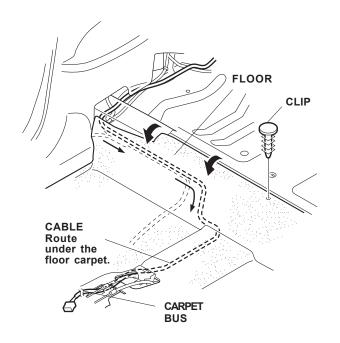
21. Route the BUS cable forward to the right front console frame along the vehicle harness.
