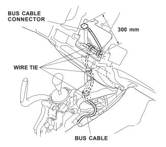
24. Along the center console area, secure the BUS cable to the vehicle harness with three wire ties.
