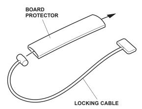
14. Insert the locking cable plate into the slot of the snowboard carrier. To carry one snowboard, insert the plate into the lowest slot. To carry two snowboards, use one of the three upper slots in the carrier.
