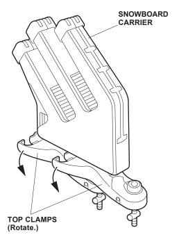
Install two board supports on the snowboard carrier.
