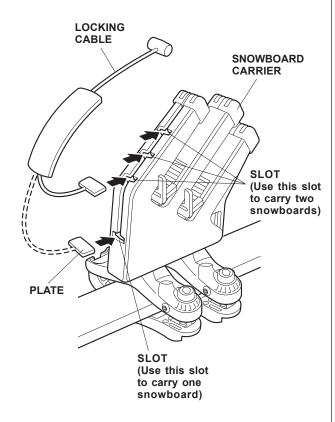
15. After loading each snowboard on the carrier, adjust it with the help of the board supports so that the top edges are level and the boards are as far down in the carrier as possible. To secure the snowboard use the key to open the covers, then insert the locking cable stoppers into the holes of the carrier covers.
