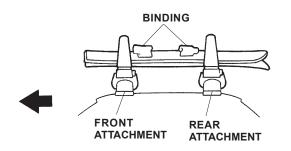
• If the bindings cannot be positioned between the front and rear attachments, install the skis with one of the bindings positioned behind the rear attachment.
