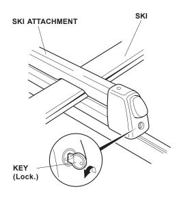
5. With the ski attached, rock the attachment in all directions to make sure it is installed securely. Adjust as necessary.
