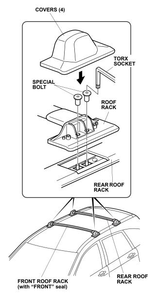
5. Reinstall the four covers on the front roof rack.
