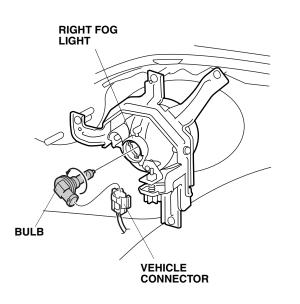
4. Install the new bulb and socket to the fog light. Use only a genuine Honda halogen light bulb of specified wattage.
