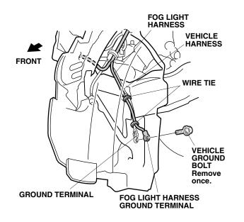
14. Secure the fog light harness to the vehicle harness using two wire ties.
