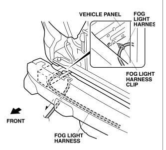
22. Secure the four remaining fog light clips to the holes in the vehicle panel.
