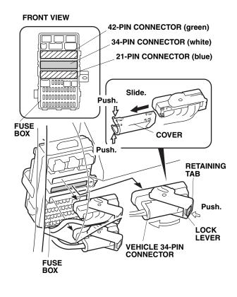
36. Insert the white and pink switch harness terminals into the appropriate cavities of the vehicle white 34-pin connector.
