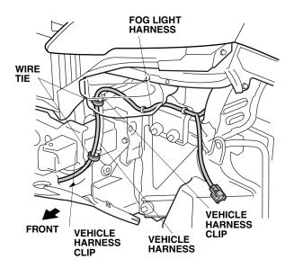
Without a Vehicle Harness: Secure the fog light harness to the vehicle panel using two wire ties with clips.
