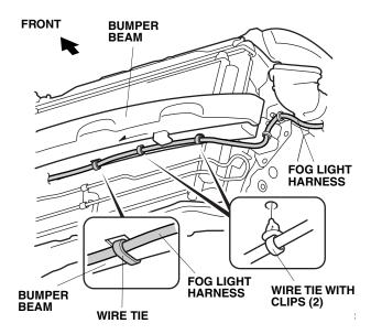
19. Using isopropyl alcohol on a shop towel, clean the bumper beam surface where the harness tape will attach.
