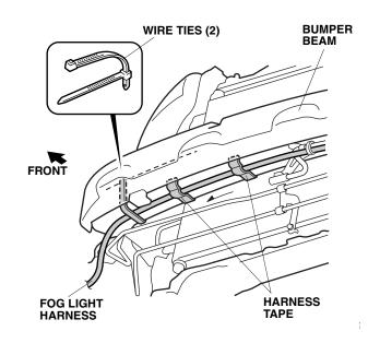
20. Continue routing the fog light harness along the bumper beam to the right side of the vehicle. Secure the fog light harness under the bumper beam using two adhesive tapes and two wire ties connected together.l 21. Attach the clip on the fog light harness to the vehicle panel.
