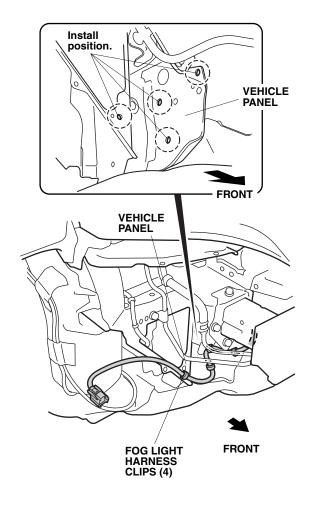
23. Reinstall the inner fender. With the help of an assistant, bring the front bumper close to the vehicle, and plug the fog light harness 2-pin connectors into the right and left fog lights. Reinstall the front bumper.
