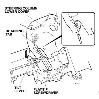
29. Remove the steering column upper cover (four retaining tabs).
