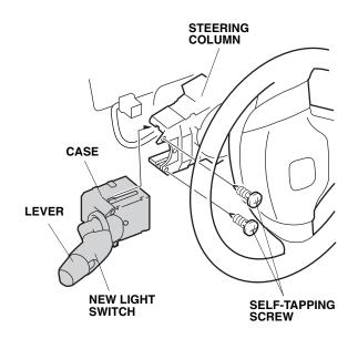
42. Plug the vehicle connector into the new light switch.
