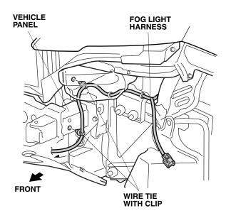
With a Vehicle Harness: Secure the fog light harness to the vehicle harness using three wire ties.
