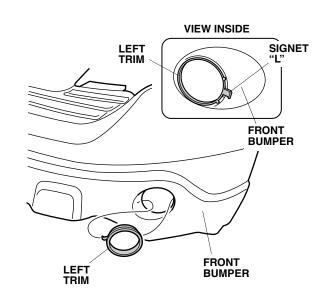
9. Install the left fog light to the front bumper using four self-tapping screws.
