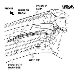
18. Route the fog light harness under the bumper beam towards the right side of the vehicle. Secure the fog light harness.
