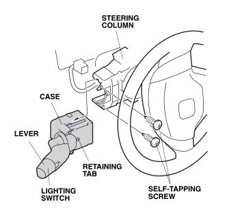
41. Install the new light switch on the steering column using the two self-tapping screws. While installing, do not hold the light switch by the lever.
