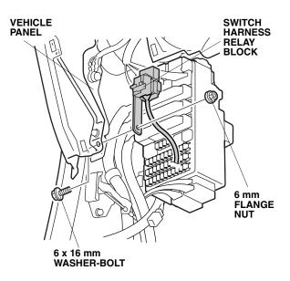
34. Plug the switch harness 2-pin connector into the vehicle harness 2-pin connector. Secure the switch harness to the vehicle harness using two wire ties.
