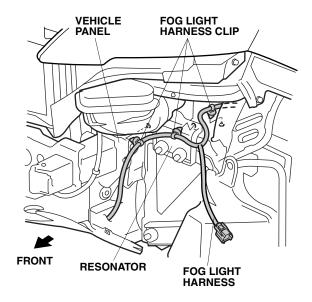
Secure the fog light harness to the front bulkhead.
