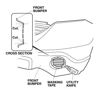
7. Using a utility knife, cut out the front bumper as shown. Take care not to damage the front bumper. After cutting, remove any burrs from the edges of the hole.
