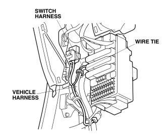
38. Secure the switch harness to the vehicle harness using one wire tie.
