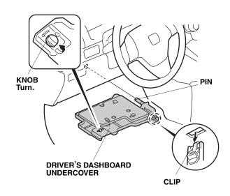
25. Remove the driver's dashboard lower cover (seven clips and two hooks).
