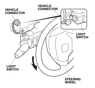
40. Remove the two self-tapping screws from the light switch. While pushing the retaining tab, slide the light switch, and remove it from the steering column. While removing, do not hold the light switch by the lever.
