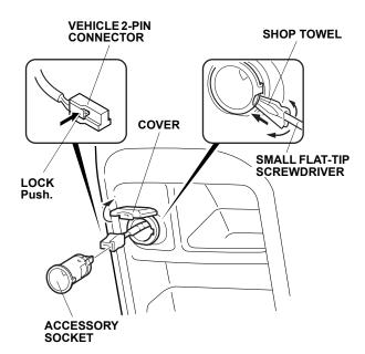
6. Pull out the accessory socket housing from the center lower cover.
