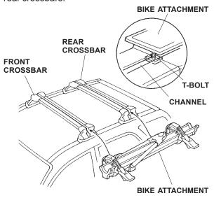
Turn and adjust the mounting lever to lock the bike attachment to the roof rack. Check for firm pressure while you push down on the mounting lever to lock it into place.
