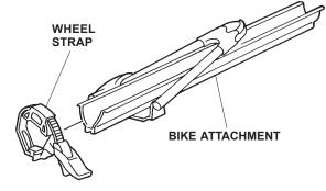
Install an end cap on the bike attachment channel by aligning the locktabs on the end cap, with the holes in the channel. Push down on the end cap until the locktabs "click" into place. Repeat on the other end.
