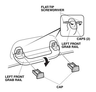
10. Using needle nose pliers, remove the left front grab rail (two clips).
