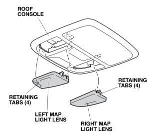
4. Remove the roof console (four bolts and unplug the vehicle connectors).
