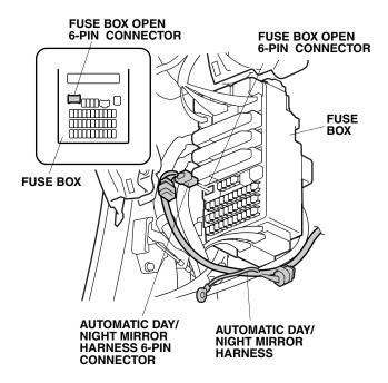
NOTE: If another accessory is already plugged into the 6-pin connector opening of the fuse box, remove the dummy connector from the 6-pin connector taped to the automatic day/night mirror harness. Plug the 6-pin connector from the other accessory harness into the
