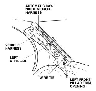
19. Route the automatic day/night mirror harness above the headliner from the left A-pillar to the middle of the vehicle.
