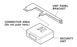
14. Without dashboard under cover: Attach the unit panel bracket to the instrument panel with two washer-screws.
