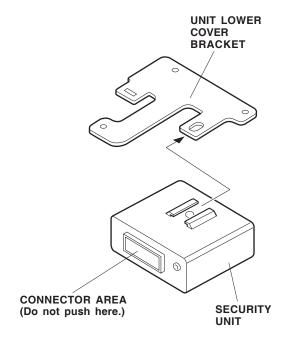
17. With dashboard under cover: Attach the unit lower cover bracket to the dashboard under cover with three self-tapping screws.
