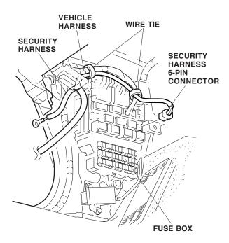
Attach the security harness to the vehicle harness with two wire ties.
