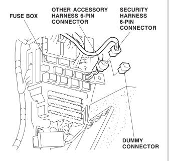
Route the ground terminal of the security harness along the vehicle harness. Remove upper bolt from the hood opener, and install the ground terminal using a new ground bolt.
