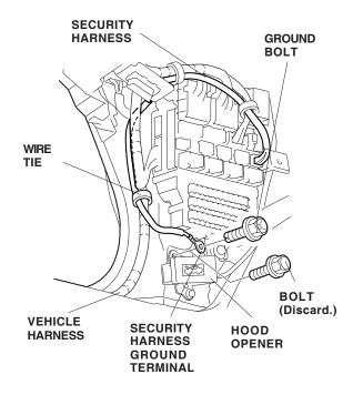
12. Attach the security harness to the vehicle harness with one wire tie.
