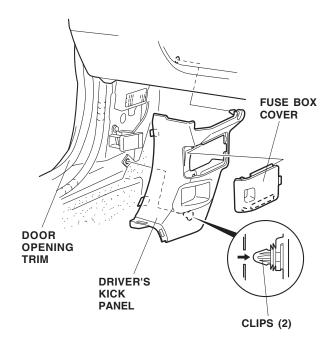
8. Remove the driver's side front door opening trim in the area shown, and remove the driver's kick panel by releasing the two clips.
