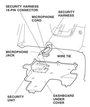
27. Attach the microphone cord to the security harness with one wire tie. Reinstall the dashboard under cover.
