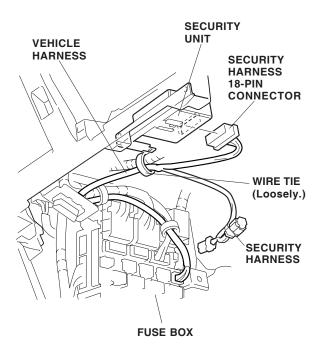
16. With dashboard under cover: Slide the security unit into the unit lower cover bracket. Do not push on the connector area.
