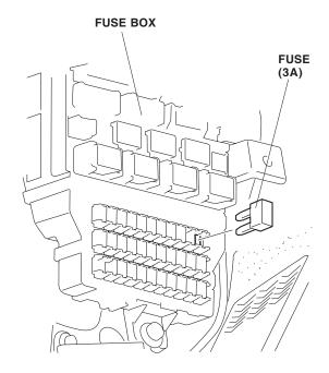
30. Attach the fuse label (OPTION FUSE 3A) over the No. 33 on the back of the fuse box cover.
