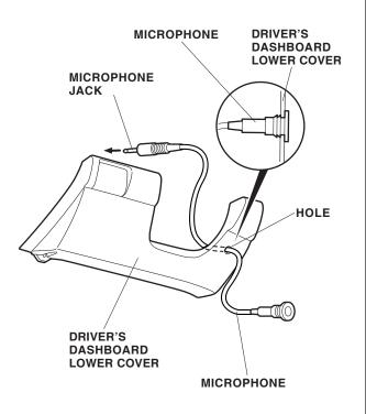
23. Without dashboard under cover: Connect the microphone jack to the security unit, and secure the microphone cord to the vehicle panel with one wire tie. Reinstall the dashboard lower cover. Fold the excess length of the microphone cord, and secure the microphone cord to the security harness with two wire ties.
