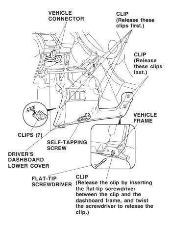
4. If equipped, remove the driver's dashboard under cover (release the three retaining clips, one pin, and one holder).
