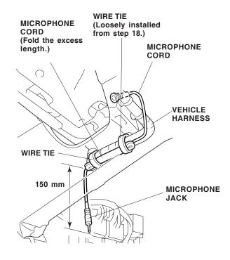
25. Attach the security harness to the vehicle harness with one wire tie.
