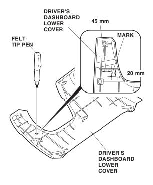
21. While wearing eye protection, drill an 8 mm hole through the felt-tip mark. First drill a 3 mm bit, then finish with an 8 mm bit. Remove all burrs.
