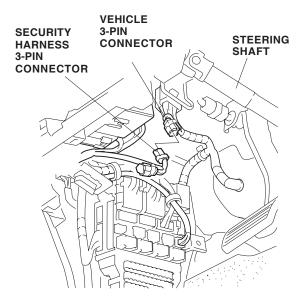
NOTE: If the 3-pin connector is already being used by another accessory, locate the 3-pin connector taped to the other accessory's harness. Remove the dummy connector from the other accessory's harness. Plug the security harness 3-pin connector into the other accessory's harness.
