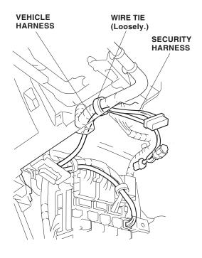
19. On the left of the steering shaft, locate the 3-pin connector blue-taped to the vehicle harness, and connect the security harness 3-pin connector to that 3-pin connector.
