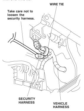
26. Plug the security harness 18-pin connector and microphone jack into the security unit.
