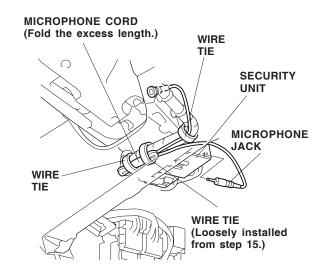
24. With dashboard under cover: Measure and fold the excess length of the microphone cord, and secure the microphone cord to the security harness with one wire tie.
