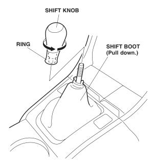
Remove the shift knob from the ring by squeezing the retaining tabs and pushing it up with long nose pliers.
