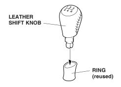
4. Install the leather shift knob on the shift lever by turning it in the clockwise direction.
