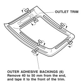
3. Position the trim pieces on the existing panels. While applying light pressure on the trim pieces, carefully remove the adhesive backings.
