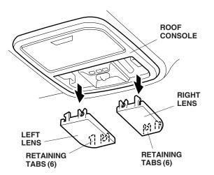
4. Remove the roof console (four bolts, and unplug the two connectors).
