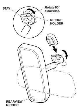
6. Replace the mirror spring. Slide the day/night mirror stay onto the mirror holder, then turn the mirror stay counterclockwise as shown.
