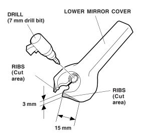
9. While wearing eye protection, drill a 7 mm hole through the existing hole on the lower cover as shown.
