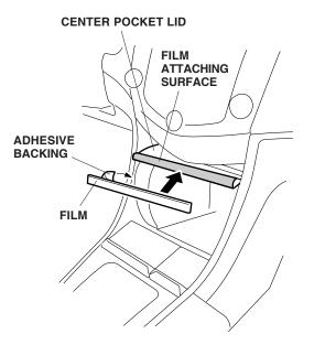
2. Remove the adhesive backing from the film, and attach it to the center pocket lid aligning the lower edge of the film with the lower end of the curved surface of the center pocket lid.
