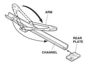
Remove the rubber bumper from the channel, and transfer it to the new location on the channel. Rotate the arm to rest against the rubber bumper. 5. Adjust the front plate to 305 mm from the end of the channel, and retighten the socket bolt.
