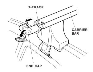
10. Remove the rubber moldings from the T-tracks of the front and rear carrier bars. Retain the rubber moldings to be installed later.
