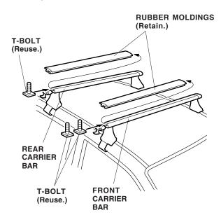
11. Slide two T-bolts into the front carrier bar, and slide one T-bolt into the rear carrier bar.
