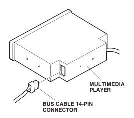
Plug the player BUS cable connector to the vehicle connector, then reinstall the player and pocket.
