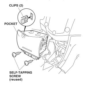
37. Reinstall the player panel using the two screws removed in step 8.
