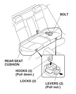
11. Remove the left side cushion (one bolt and two hooks).
