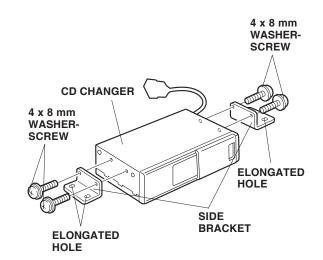
14. Position the CD changer on the CD changer bracket, then install the four flange nuts. Tighten the flange nuts securely.
