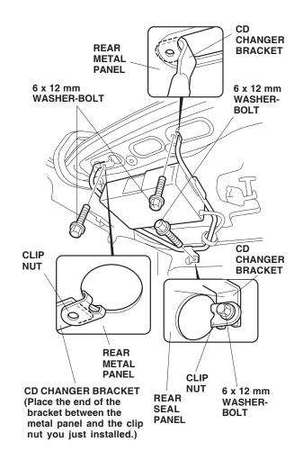
Loosely install the 6 x 12 mm washer-bolt to the rear seat panel first. Secure the CD changer bracket to the metal panel with the remaining two 6 x 12 mm washer-bolts. Tighten all three bolts.
