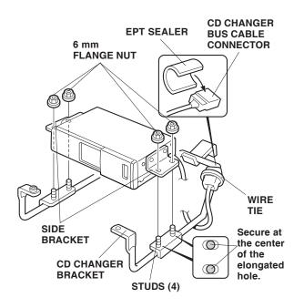
15. Wrap the CD changer BUS cable connector with one EPT sealer, then secure it to the CD changer bracket with one wire tie.
