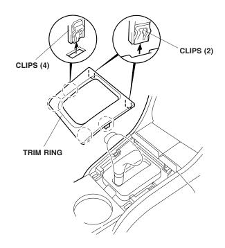
4. Wiggle and then pull up on the cup holder to release the six clips, then remove the cup holder.
