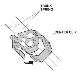
14. With an assistant holding the trunk lid open, remove the old trunk springs from the trunk hinge arms using the special tool. Wear gloves to protect your hands, and pull the special tool slowly and carefully toward you.
