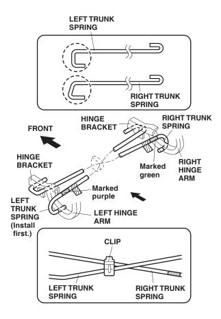
16. Reinstall the center clip on the trunk springs.
