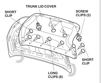
2. Remove the two clips that secure the vehicle harnesses to the trunk lid, and tape the harnesses to the trunk lid with masking tape.
