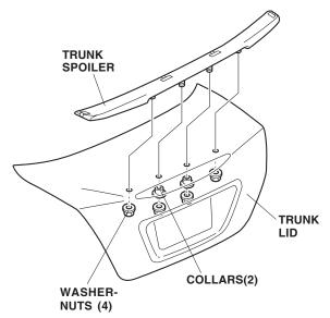
8. Fit the trunk spoiler into position on the trunk lid by inserting the four studs into the holes in the trunk lid. With an assistant holding the trunk lid open, install the two collars and four washer-nuts, but do not tighten them yet. 9. While aligning the trunk spoiler with the trunk lid, carefully remove the adhesive backings from both sides. Hold the spoiler firmly against the trunk lid with the palm of your hand.
