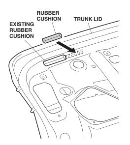
18. Remove the adhesive backing from the rubber cushion, and attach it to the inside panel of the trunk lid next to the existing rubber cushion. After attaching it, use the palm of your hand to hold pressure against it for 30 seconds. Repeat on the right side. Then go to step 23.
