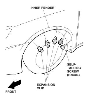
Pull the inner fender down, and position the left front fenderwell trim between the inner fender and the fender flange. Align the fenderwell trim with the front bumper as indicated by the arrow.
