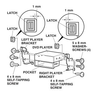
67. Position the DVD player and pocket on the left and right player brackets, and install four 5 x 8 mm washer-screws from the player kit, and the two 4 x 8 mm self-tapping screws from the player attachment kit.
