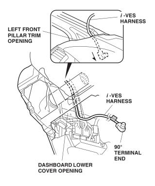
31. Continue routing the  $90^{\circ}$  end of the *i*-VES harness from the dashboard lower cover opening to the pocket opening on the driver's seat side.
