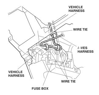
46. Continue to secure the *i*-VES harness to the vehicle harness with the three wire ties in the areas shown.
