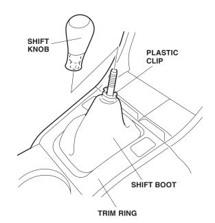
• *With locknut:* Loosen the lock nut and remove the gearshift knob.
