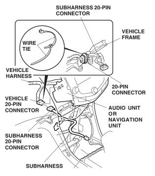
48. Secure the connected 20-pin connectors to the vehicle frame with two wire ties.
