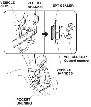
53. Using diagonal cutters, cut and remove the vehicle clip. Wrap one EPT sealer around the vehicle harness.
