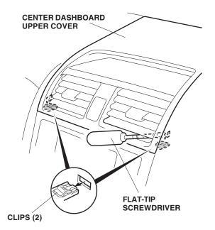
• Push in on the hazard warning switch bottom. Carefully insert a flat-tip screwdriver into the slot at the bottom of the hazard warning switch, then pry up the middle portion of upper panel by releasing the center clip.
