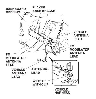
59. Wrap the FM modulator antenna lead and vehicle harness you removed with one wire tie with clip, and push the wire tie with clip into the hole in the player base-bracket.
