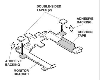
39. Using isopropyl alcohol on a shop towel, clean the vehicle frame where double-sided tapes will attach. Remove the adhesive backings from the double-sided tapes, position the monitor bracket on subbracket A and install the two screws to secure the interior light.
