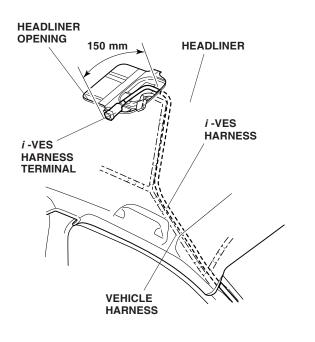
35. Using isopropyl alcohol on a shop towel, clean the area where the cushion tape will attach. Secure the *i*-VES harness to the headliner with the three cushion tapes along with the vehicle harness.
