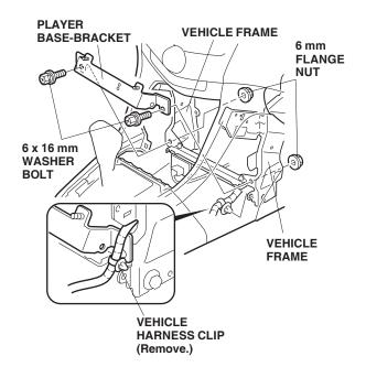
• *Without YAW sensor:* Install the player basebracket to the vehicle frame, then install the two 6 mm flange nuts while holding the bracket firmly against the vehicle frame.
