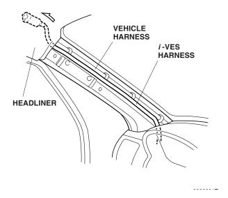
34. Continue routing the *i*-VES harness to the rear along the vehicle harness, and out the opening in the headliner, so that the distance between the headliner opening and end of the *i*-VES harness is 150 mm.
