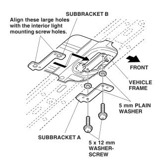
37. Install the two 5 mm plain washers and the subbracket A with the two 5 x 12 mm washer-screws.
