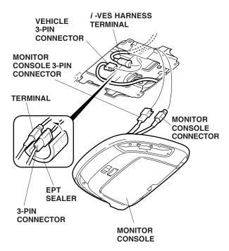
42. Wrap one EPT sealer around the terminals and 3-pin connectors.
