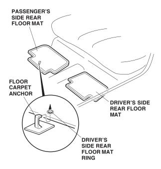
4. Install the passenger's side rear floor mat by placing the ring in the floor mat around the anchor on the floor carpet.
