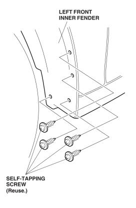
Position the left front splash guard on the left front inner fender, and install the four self-tapping screws you just removed.
