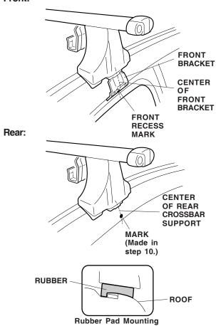
13. Set the rubber pads on the roof as shown
