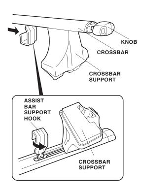
Adjust the distance between the two crossbar supports. Using the measurements on the crossbars, open the lock arm, and slide the supports in or out until the correct measurement is obtained. Close the lock arms to secure the crossbar supports.
