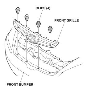
3. Inside the front grille, cut off the two pins, and remove the push nuts and the old "H" emblem.
