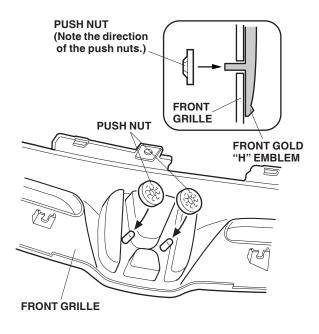
6. Reinstall all removed parts. Check that the clips are installed securely.
