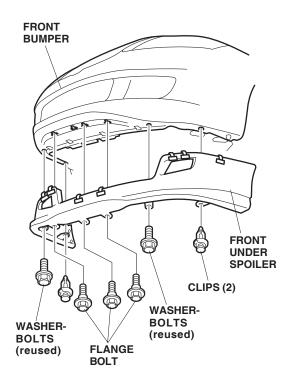
7. While holding pressure on the front under spoiler against the front bumper, install the two self-tapping screws on each side. Do not tighten the self-tapping screws yet.
