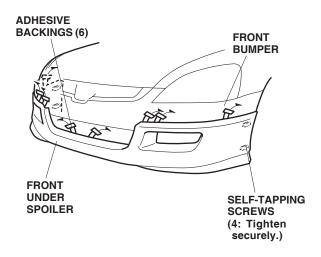
9. Tighten the four self-tapping screws temporarily installed in step 7.
