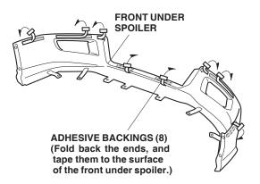
Using isopropyl alcohol on a shop towel, clean the front bumper where the front under spoiler will attach. 6. Position the front under spoiler on the front bumper. Then install three flange bolts, two new clips, and the two washer-bolts removed in step 2.
