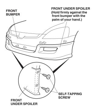
8. Starting in the center and working your way around the sides, hold light pressure on the front under spoiler, and carefully remove the adhesive backings from the front under spoiler. Using the palm of your hand, hold the front bumper spoiler firmly against the front bumper for 30 seconds.
