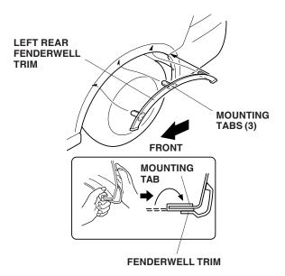
9. Fill the cavity of the inner protector with dishwashing soap and water-solution as a lubricant, then drive the inner protector over the fender flange and fenderwell trim using a rubber mallet. Note the direction of the inner protector.
