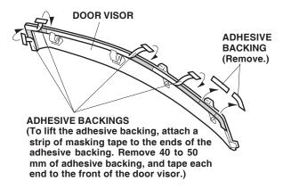
11. Attach a strip of the masking tape to the ends of the remaining adhesive backings, and remove 40 to 50 mm from the end. Fold back the ends, and tape the ends to the front of the door visor. Note the direction of the adhesive backings. 12. Insert the front tab under the door mirror base.
