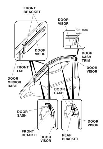
13. Adjust the location of the door visor so that the clearance between the door visor and door sash trim is 8.5 mm at the rear of the door. There should be no clearance between the front tab and the door visor.
