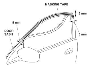
7. Using isopropyl alcohol on a shop towel, clean the door sash inside the masking tape. Also clean the door sash trim inside the masking tape with isopropyl alcohol by rubbing the surface with force at least 6 times both ways.
