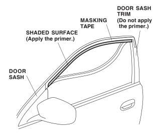
Attach the masking tape to the door visor in the area shown.
