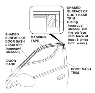
8. While wearing gloves, apply the primer to the door sash below the masking tape. Do not apply the primer to the door sash trim. Wipe up excess primer at once. Allow the primer to dry for at least 3 minutes, then remove the masking tape.
