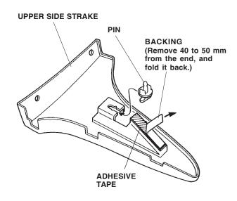
17. Remove 40 to 50 mm of the backing from the adhesive tape, and fold it back as shown.
