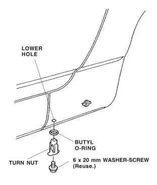
10. Position the lower side strake on the body, and reinstall the 6 x 20 mm washer-screw. Secure the back of the side strake with two clamps. If necessary, remove any excess undercoating so the clamps attach securely. Tighten the 6 x 20 mm washer-screw and the clamps securely.
