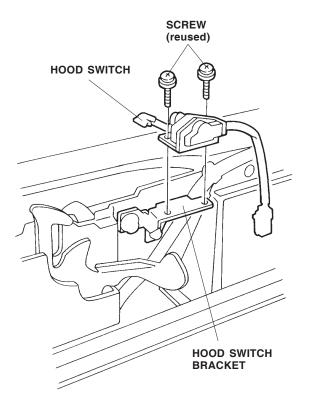
9. Route the hood switch wire harness as shown, and secure it to the vehicle harness with two short wire ties.
