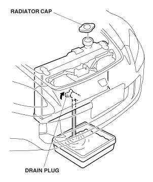
3. Locate and remove the engine block drain bolt and washer. Coolant remaining in the engine jackets flows out of the bolt hole when the bolt is removed. (Retain the bolt in case the block heater is removed.)
