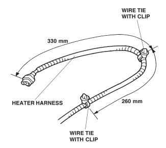
6. Plug the connector of the heater harness into the engine block heater.
