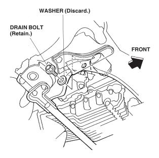
Install the new aluminium washer and the engine block heater into the bolt hole using a 24 mm socket and a torque wrench. Torque the engine block heater to 60 N·m (44 lb-ft).
