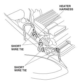
11. Secure the heater harness to the vehicle harness with four short wire ties in the areas shown.
