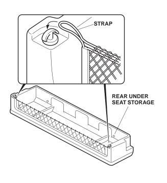
6. Position the rear under seat storage on the floor mat, and align the holes in the rear under seat storage with the holes in the brackets. Secure the seat storage with the two knob bolts.
