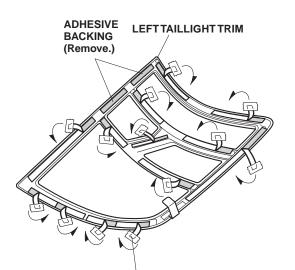
ADHESIVE BACKINGS (13) Peel back 1 1/2 to 2 in. (3-5 cm) of the adhesive backing strips and attach them to the front of the trimwith masking tape.
