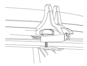
6. Slide the buckle on the attachment strap into the clip on the base.
