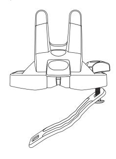
2. Position the base on the crossbar. Loosely install a bolt and knob as shown.
