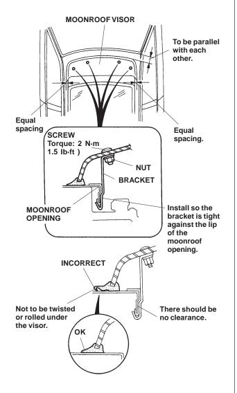
10. Torque the screws to 2 N·m (1.5 lb-ft), alternating between sides. To prevent damage to the resin nuts, do not over-tighten the screws.
