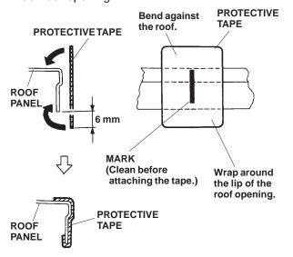
7. Place the two front brackets A into position by sliding them along the lip of the roof opening. Set the moonroof visor on the vehicle roof, in front of the moonroof opening, and adjust its position so the holes in the visor are aligned with the protective tapes.
