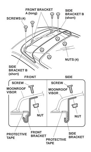
While holding the visor in place, install the four screws, four nuts, and four brackets A and B with the end of each bracket hooked to the lip of the moonroof opening. Do not tighten the screws yet. 9. Position the moonroof visor with equal spacing on all sides. Check that the rubber seal is not twisted or rolled under the visor.
