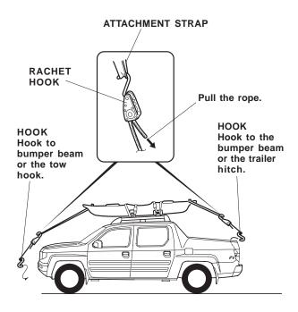
13. To loosen the rope, push up on the ratchet strap lever, then pull on the rope.
