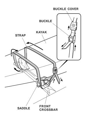
8. Route the strap under the rear crossbars, and around the kayak as shown. Slide the buckle cover away from the buckle, route the strap through the buckle, and tighten the strap. Slide the buckle cover back over the buckle.
