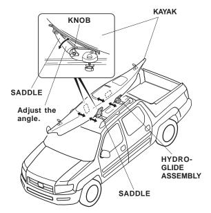
Slide the kayak forward or backward until it's level with the roof. If necessary, loosen the knob on each saddle and adjust the saddle angle to fit snugly against the kayak. Tighten each knob securely. 6. Route each strap with buckle through the buckle cover with the ribbed end facing up.
