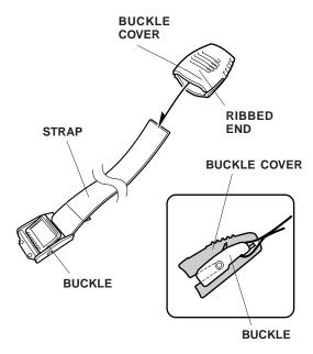
7. Route the strap under the front crossbars, and around the kayak as shown. Slide the buckle cover away from the buckle, route the strap through the buckle, and tighten the strap. Slide the buckle cover back over the buckle.
