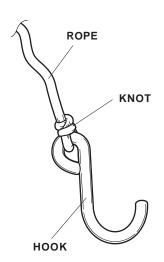
Route the other end of the rope through the bottom of a rachet hook in the direction shown, and turn the spool until the rope end comes out of the rachet.
