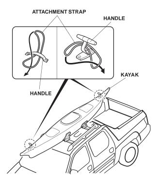
12. Attach one ratchet hook to the front attachment strap and one rachet hook to the rear attachment strap. Attach the front hook to the front bumper beam or to the tow hook. Attach the rear hook to the rear tie-down anchors in the bed. Secure the kayak to the vehicle by pulling the rope through the ratchet hooks.
