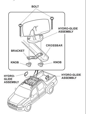
Rest the front of the kayak on the hydro-glide assemblies. Standing behind or alongside the kayak, lift up the rear end portion of the kayak and push it forward, sliding on the hydro-glide assemblies and saddles. Make sure the kayak reaches the front saddles before you lower it.
