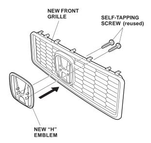
5. Position the new front grille on the front bumper, and install it with the eight retaining tabs.
