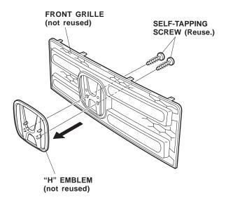
4. Slide the pins from the new "H" emblem into the holes in the new front grille, and install the two self-tapping screws you just removed.
