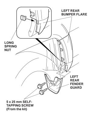
30. Install the left rear fender guard on the inner fender with one clip (from the kit).
