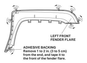
5. Align the ends of the front fender flare with the front end of the front fender, and bend the mounting tabs around the fender flange. Reinstall five expansion clips through the holes in the fender flare and fender flange.
