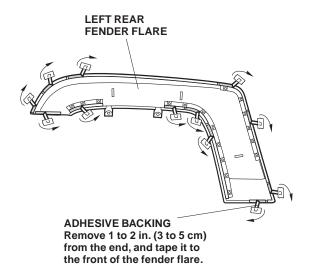
21. Align the ends of the rear fender flare with the rear end of the rear fender, and bend the mounting tabs around the fender flange. Install two clips from the kit through the holes in the fender flare and fender flange.
