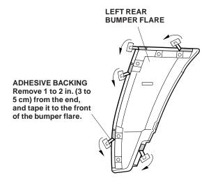
26. Position the left rear bumper flare on the rear bumper and install the two self-tapping screws removed in step 23 through the rear bumper. Do not tighten the self-tapping screws yet.
