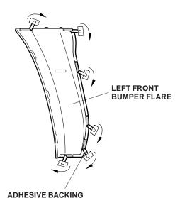
13. Position the left front bumper flare on the front bumper and install the three 5 x 20 mm self-tapping screws (from the kit) through the front bumper. Do not tighten the self-tapping screws yet.
