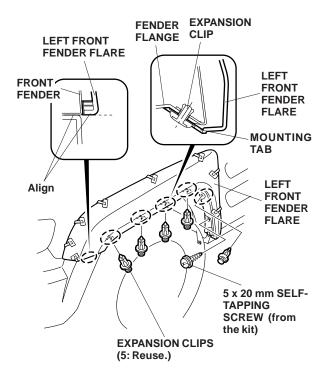
6. Install one 5 x 20 mm self-tapping screw (from the kit). Do not tighten the self-tapping screw yet.
