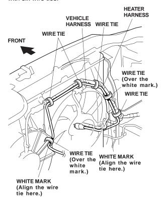
8. Continue routing the heater harness along the vehicle harness and down to the bumper grille opening. Attach the protective cap to the bumper grille, and plug the heater harness connector into the protective cap.
