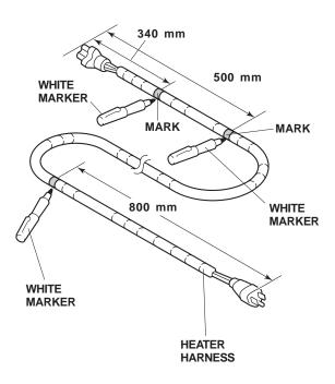
Plug the heater harness connector into the engine block heater, and secure the heater harness to the vehicle harness with one wire tie at the white mark.
