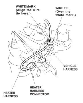
7. Route the heater harness over the fan shroud and along the vehicle harness. Secure the heater harness to the fan shroud and vehicle harness with six wire ties.
