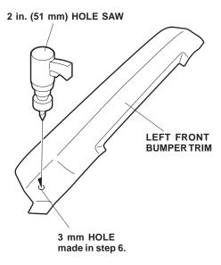
13. Remove the adhesive backing from the left front bumper trim, and attach one EPT sealer to the inside edge of the left front bumper trim.
