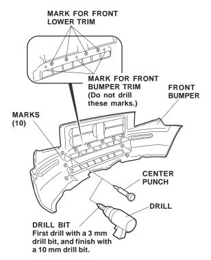
11. Get the left front bumper trim. While wearing eye protection, drill a 3 mm hole through the mark on the inside of the left front bumper trim.
