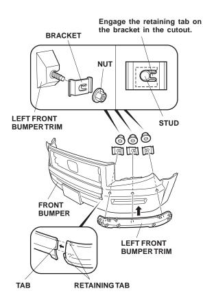
19. While holding light pressure on the trim, carefully remove the adhesive backings from the trim. After removing the adhesive backings, hold the trim firmly against the front bumper with the palm of your hand for 30 seconds.
