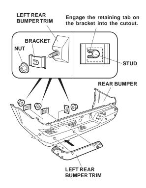
31. Align the upper line of the bumper trim with the masking tape. While holding light pressure on the trim, carefully remove the adhesive backings from the trim. After removing the adhesive backings, hold the trim firmly against the rear bumper with the palm of your hand for 30 seconds.
