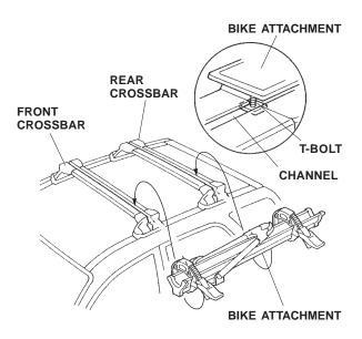
Turn and adjust the mounting levers to lock the bike attachment to the roof rack. Check for firm pressure while you push down on the mounting lever to lock it into place.
