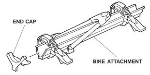
Turn the three mounting levers on the bike attachment to loosen them.
