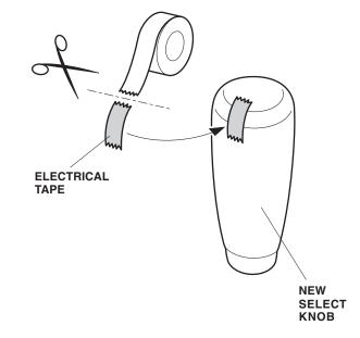
Thread the new select knob onto the select lever 9 to 10 turns using the tape as reference. Do not overtighten the select knob.
