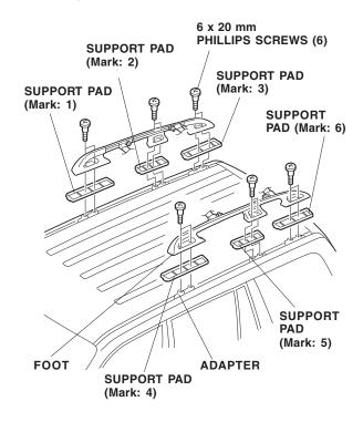
11. Rock the roof rack in all directions to check that it is mounted securely without play or rattle.
