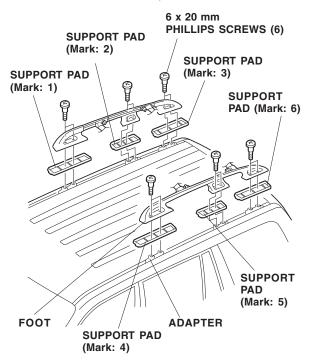
Set the rack over the support pads and onto the adapter blocks (short crossbar to the rear), and adjust the left side rail in-or-out until you can install the 12 Phillips screws into each adapter block. Torque the Phillips screws to 7 to 10 N⋅m (5 to 8 lb-ft).
