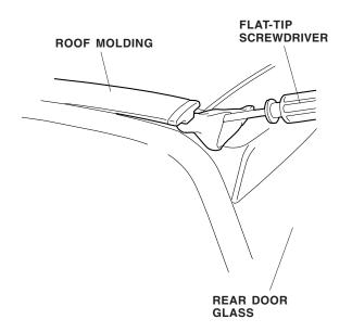
2. Remove the roof moldings by carefully pulling them upward.
