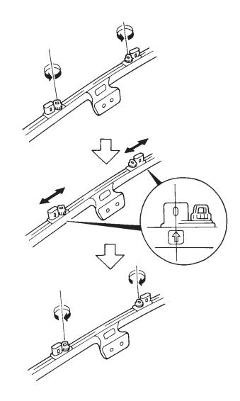
8. Insert the crossbars into the right side rail in the direction shown; install the two Torx self-tapping screws into each side rail. Insert the crossbars into the left side rail, and install two Torx self-tapping screws and nylon washers into each elongated side rail. Tighten all Torx screws securely.
