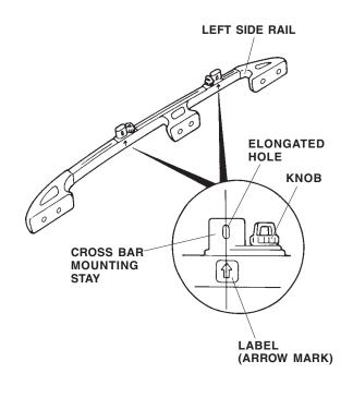
7. If any holes are not aligned, loosen the knob and slide the mounting stay until the hole is aligned with the arrow mark. Retighten the knob securely.
