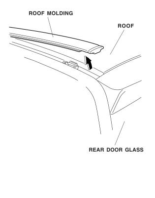
Using long-nose pliers, remove the eight retaining clips (four on each side) from the stud bolts. Discard four of the clips.
