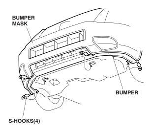
13. Attach the four hooks to the bottom edges of the bumper grille.
