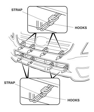
14. Attach the four hooks to the bottom edges of the lower bumper grille.
