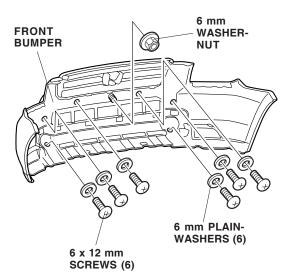
8. Reinstall the front bumper. Make sure that all clips and retaining tabs are attached properly.
