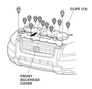
Remove the front bumper (five clips, two selftapping screws and four bolts). To prevent damage, rest the bumper on a blanket.
