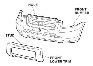
7. Secure the front lower trim to the front bumper with six 6 x 12 mm screws and six 6 mm plainwashers. Install the 6 mm washer-nut on the end of the stud, and tighten it securely.
